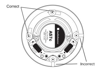
With the grill removed, place the speaker in the ceiling opening. Make sure that the speaker wire is not hanging against the speaker where it can vibrate and rattle as the speaker reproduces your music.
